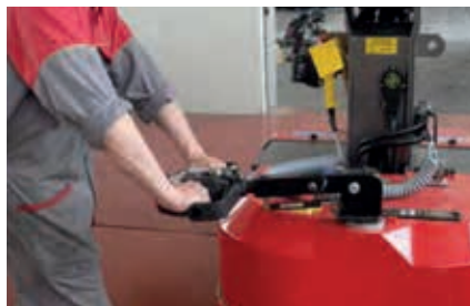
Power assisted steering tiller with 180° rotation for max. maneuverability
