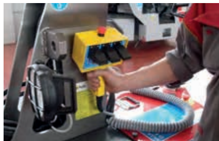
Wired remote for boom and winch
