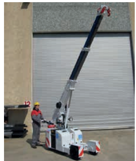
Fully hydraulic telescopic boom
