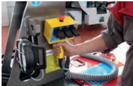
Wired remote for boom and winch
